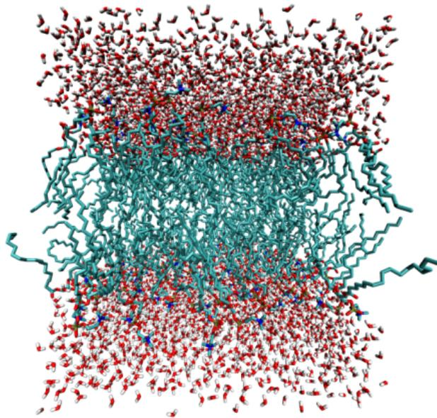
– simulation of a DOPC bilayer in water – Berger FF for the lipid
